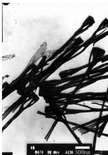
Figure 2. The TEM morphology of haematite nanowires.
